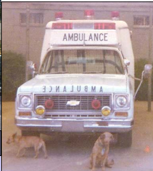
1970 TYPE I CHEVY 3500 SINGLE REAR WHEELS. FIBERGLAS MODULANCE BUILT BY MODULAR AMBULANCE CORP GRAND PRAIRE TX. 454 CU GAS BURNER OPERATED BY AMBULANCE SERVICE OF BR. TOP IN 125 MPH AT 5 MPG OR LESS.
